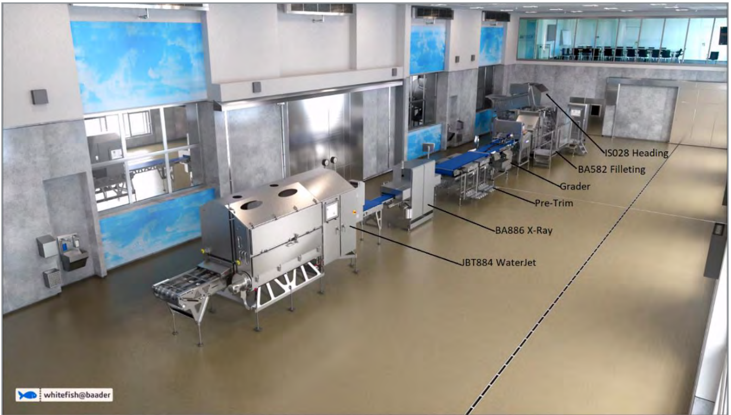
Figure 25. Conceptual drawing of Baader whitefish processing line at the Baader demonstration facility in Lubek, Germany (Source: Baader Canada)
