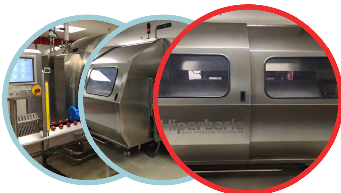
Figure 26. NC Hiperbaric Wave 6600 55L Horizontal High Pressure Processing System installed at the Fisheries and Marine Institute of Memorial University of Newfoundland
